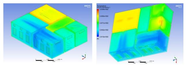
**Figure 7. Graphical representation of the temperature field** Source: compiled by the author
